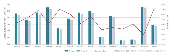
Figure 1: Comparison of daily energy yield of N-type and P-type modules
