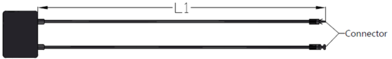
Fig. 12 (1) The full-cell module junction box
