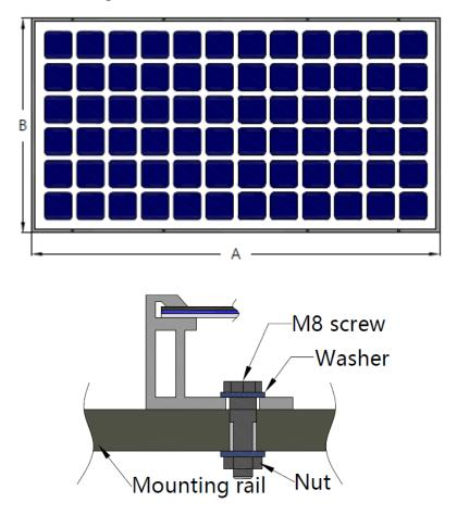
Figure 2: The mounting method of bolts for Dual glass modules with frame
