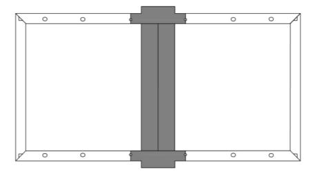
Figure 5: PV module installed with bolt fitting method (NEXTracker)
